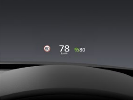
Active Driving Display is projected onto the windscreen in full colour, displaying trip information in your line of sight.
